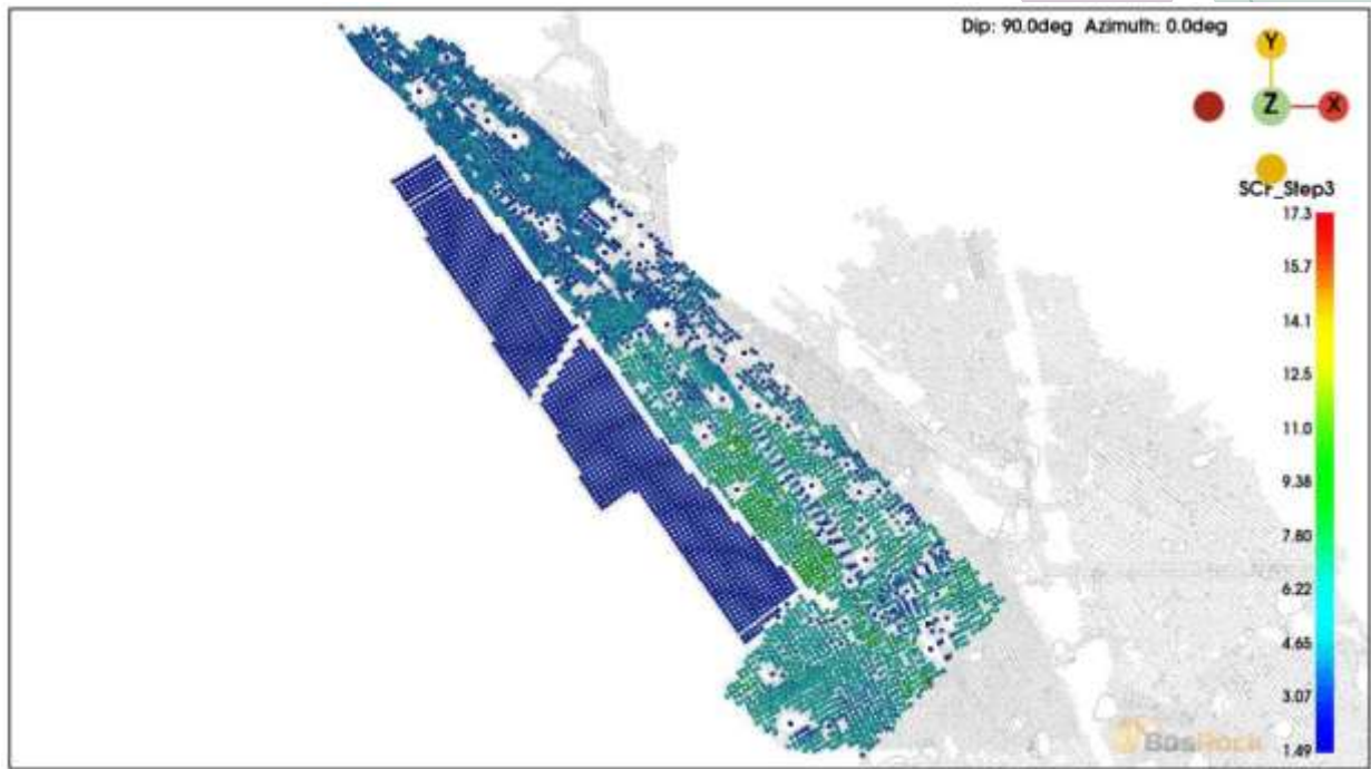
FIGURE 34: CALCULATED STRESS CONCENTRATION FACTOR FOR EACH PILLAR
